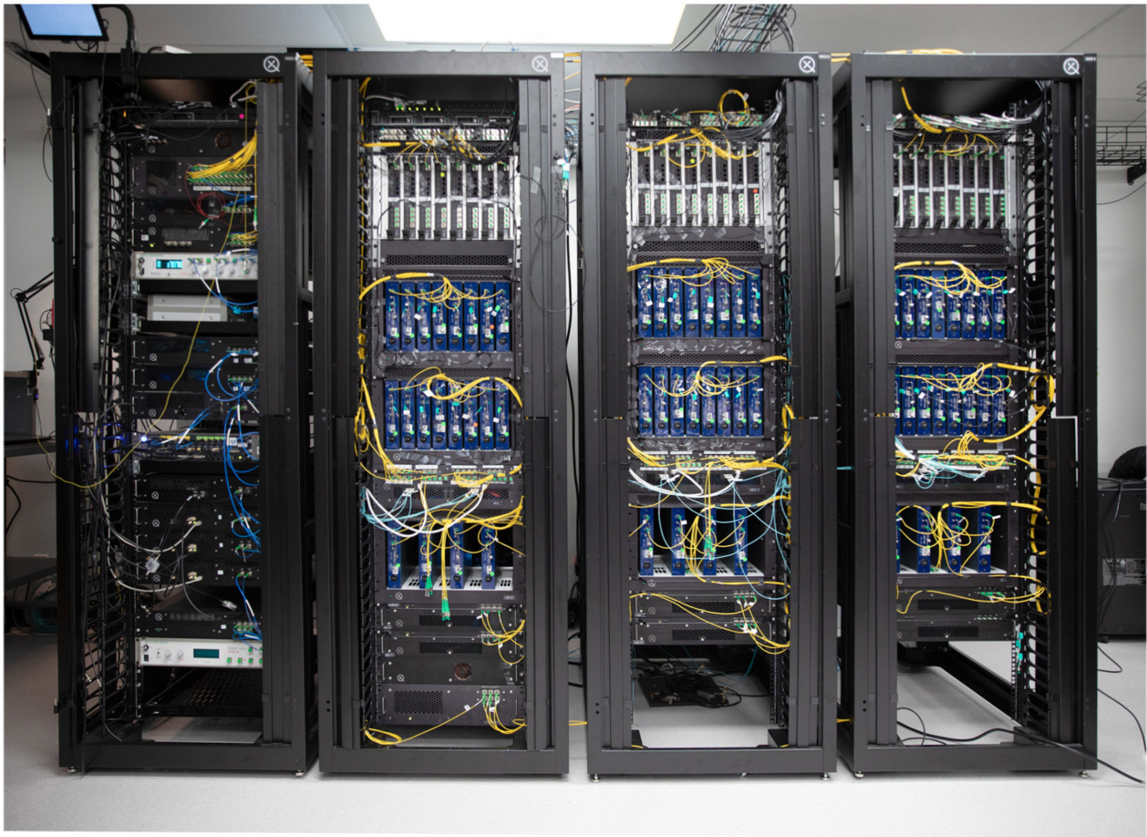
Extended Data Fig. 1 | Photograph of the Aurora system. The entire system, apart from the cryogenic detection array, fits into four standard 19-inch server racks and is fully operated using a single server computer.
