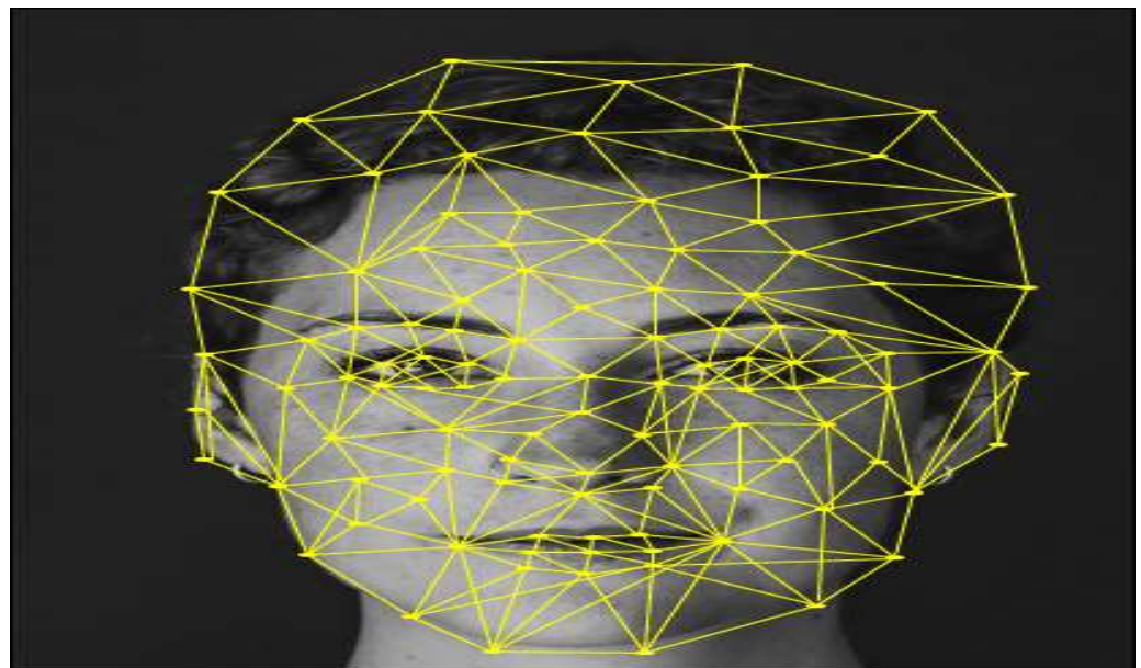
Figure 2. Polygonal template of human face. A face is made up of a number of triangles, each of which is warped to adjust the overall shape of the face [15].
