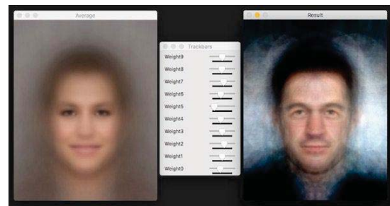
Fig4-The mean image (Left). A new face eigenface (Rights) with different weights (Center).
